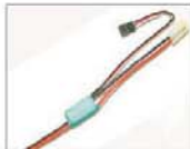
■ 521010 Electronic Speed Controller 18A
