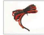
■ Silicone Wire Black & Red 612821 1M O/D:2.6mm (16AWG) 612801 1M O/D:3.2mm (14AWG) 612811 1M O/D:3.8mm (12AWG) For All Electric Models
