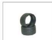
■ 253408 Tires ID61mm W38mm OD72mm For 7000 Series Car
