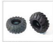
■ 253405 Rubber Tires 2.2"X2.5" ID61mm W59mm OD124mm For 5000/7000 Series Car
